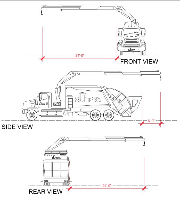
NOTE: SERVICE TRUCK CRANE REACH SPECIFICATIONS VARY BETWEEN TRUCK MANUFACTURES. THE ABOVE NOTED REACH DIMENSIONS ARE APPROXIMATE AND ARE TO BE TAKEN AS A GENERAL GUIDELINE.
